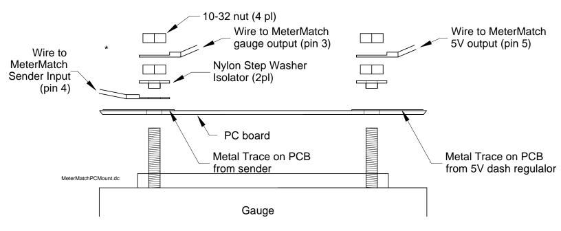
\* Note: Alternatively, the fuel sender wire can be cut under the dash, and each cut end connected to MeterMatch terminals directly. This removes the need for isolation at the back of the gauge for this terminal.
