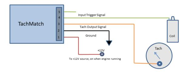
A current-driven tachometer is connected this way:
