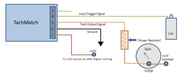
A Vintage Tach is connected this way – remember the need for a ground wire from the negative terminal of the tachometer (*Note*: to prevent damage to your tachometer, don't install the wire to the tach until the jumper, calibration potentiometer and cyl-switches are set as described on the following pages):
