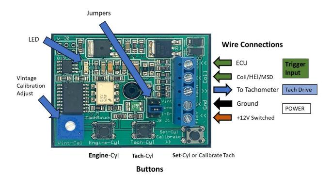
The LED illuminates when power is applied, but goes out when the engine is running, as an indication that triggering is occurring. It is also used for setting the engine and cylinder count.
