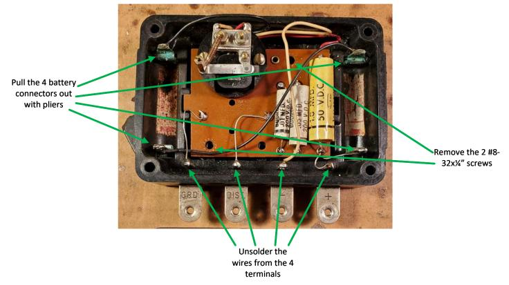
At this point the guts can be removed from the EB transmitter case:
