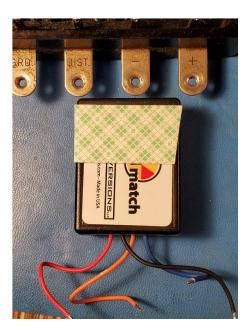
Mount the TachMatch Converter case to the rear two mounting bosses inside of the bottom of the EB case:
