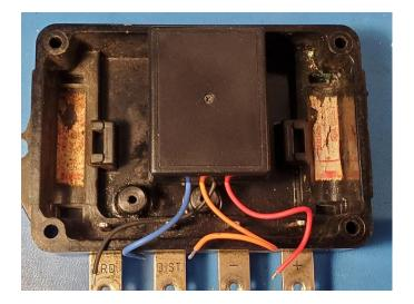
Solder the Black wire to the "GND" terminal, the Blue wire to the "DIST" terminal, the Orange wire to the "-" terminal and the Red wire to the "+" terminal:
